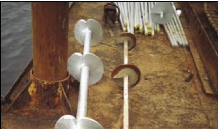
Round and square visual comparison of lead sections on a marine breakwall project – tie-back anchors
